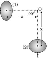
Two very small identical circular loops, (1) and (2), carrying equal currents I are placed vertically (with respect to the plane of the paper) with their geometrical axes perpendicular to each other as shown in the figure. Find the magnitude and direction of the net magnetic field produced at the point O.
