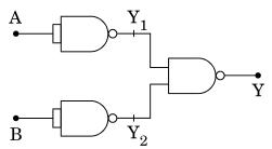
Identify the equivalent gate represented by the circuit shown in the figure. Draw its logic symbol and write the truth table.
